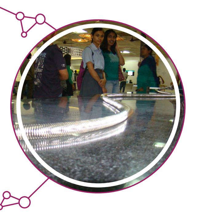
dent waves and the reflected waves interfere to produce standing waves. How many standing waves can you create? By measuring the length of the spring, the frequency with which you oscillate it, and counting the number of nodes, can you find the speed of this wave?
